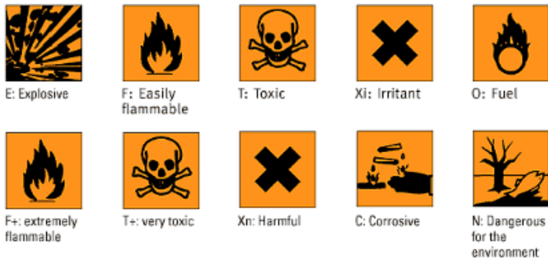
Fig. 6.13.2: Chemical hazard safety signs
