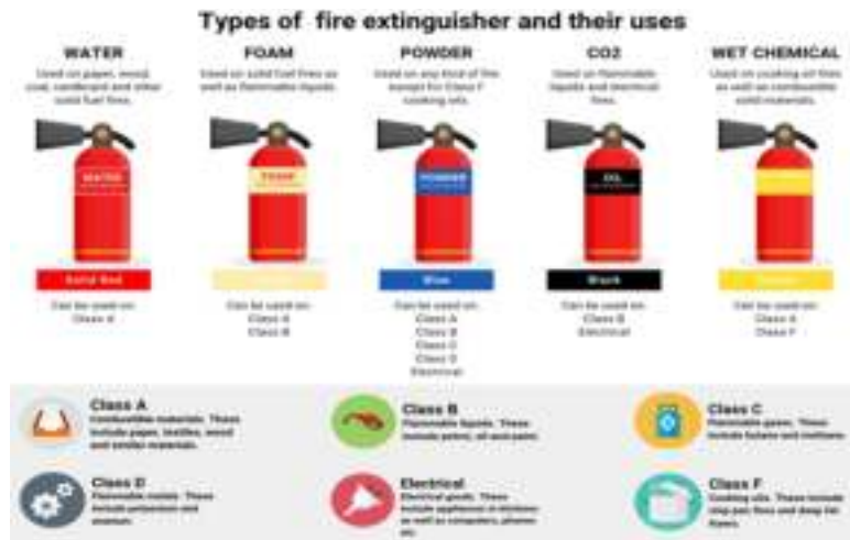
Fig. 6.7.1: Types of fire extinguishers
